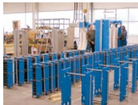
In the final assembly area for small and medium-sized PHE units
